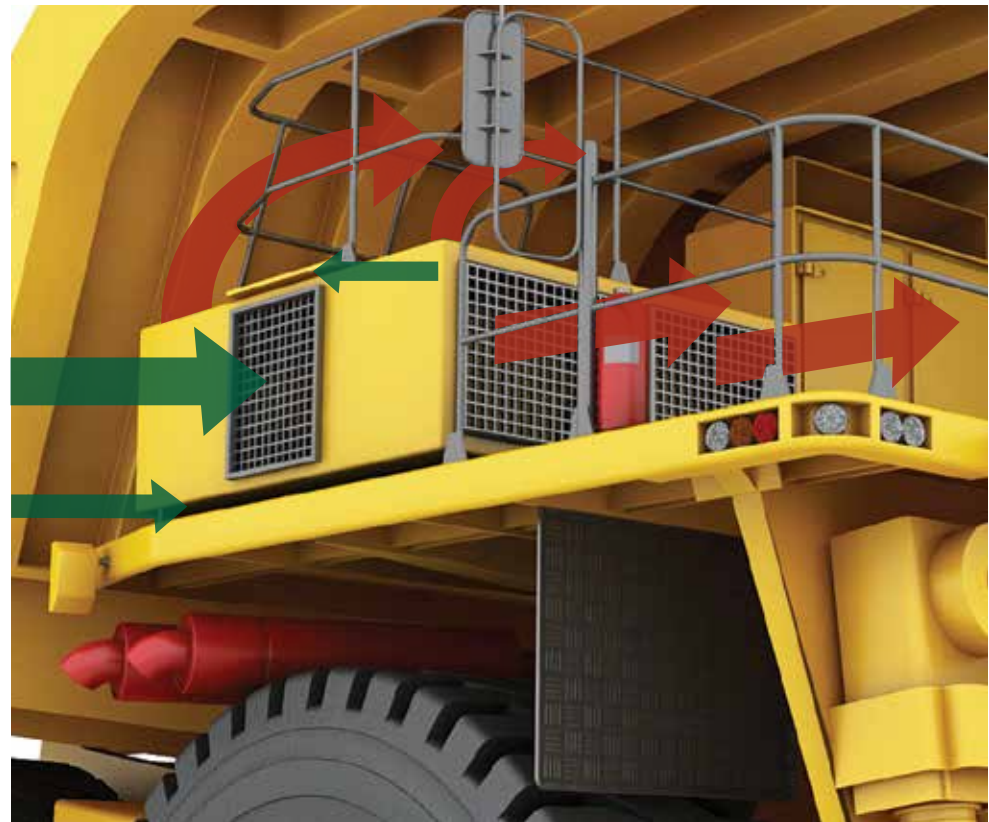
The space limitation inherent with the current OEM grid hatch design reduces air intake and allows hot, discharged air to be recirculated, which is problematic for vane axial fan applications.
